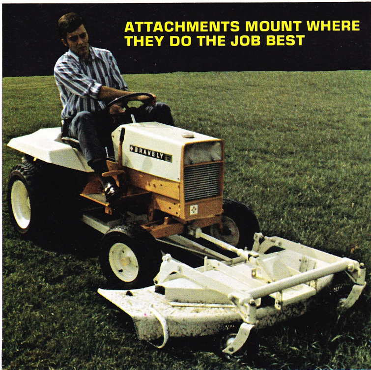
Front-mounted 50 inch Rotary Mower—all-gear-driven to single horizontal belt—carried from rear axle for maximum maneuverability and smooth cut.
