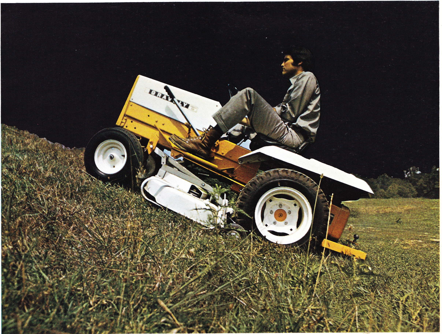
Gravely 450 16.5 hp Riding Tractor with 50 inch Rotary Mower. Two-cylinder, silk-smooth engine, special wide-tread, deep-frame design for power and stability.
