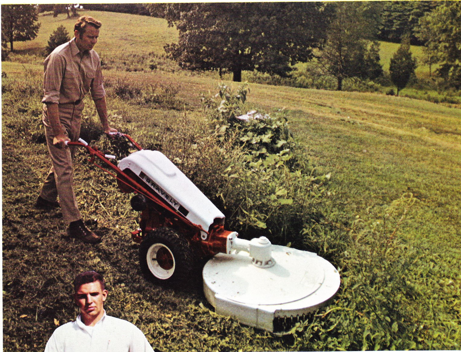
Gravelly Custom Convertible 7.6 with all-gear-drive 30 inch Rotary Mower
