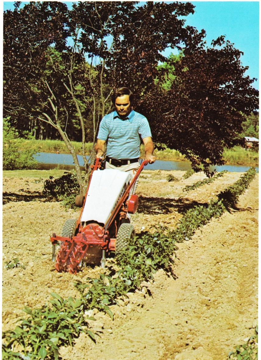
Gravely 7.6 hp Convertible Tractor with Toolholder, 5 Steel Cultivating Tools
